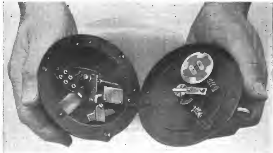
Left—Switch cover as it appears on cowboard. Right—Inside of switch showing the vibrator employed for the secondary ignition and the details of the selecting and reversing switch which gives either main or secondary ignition and-reverses the direction of the current with each click of the ratchet
